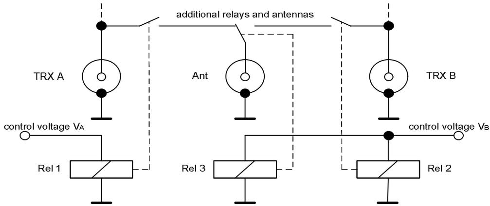
Picture 2: Adding relay 3 doubles the insulation to around 60-70 dB (depending on relays used)
