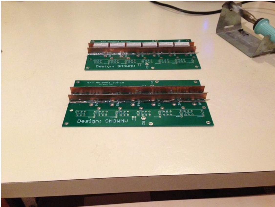
Picture 5: HF relays PCB with copper stripes between relays to increase insulation
