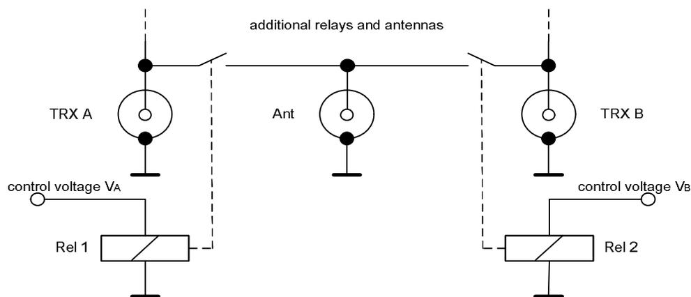
Picture 1: Simple relays circuit to use two radios on one antenna without protection against simultaneous connection.
