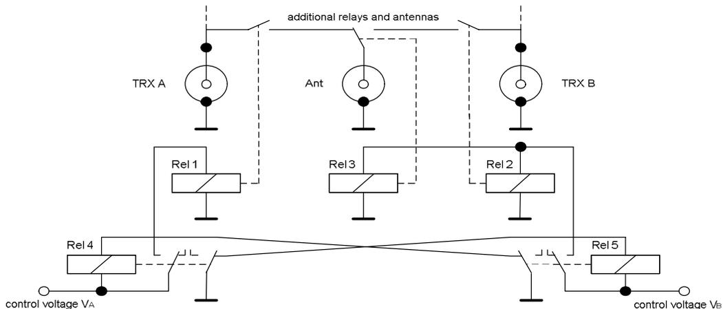
Picture 3: electromechanical interlocking for a 6x2 antenna switch
