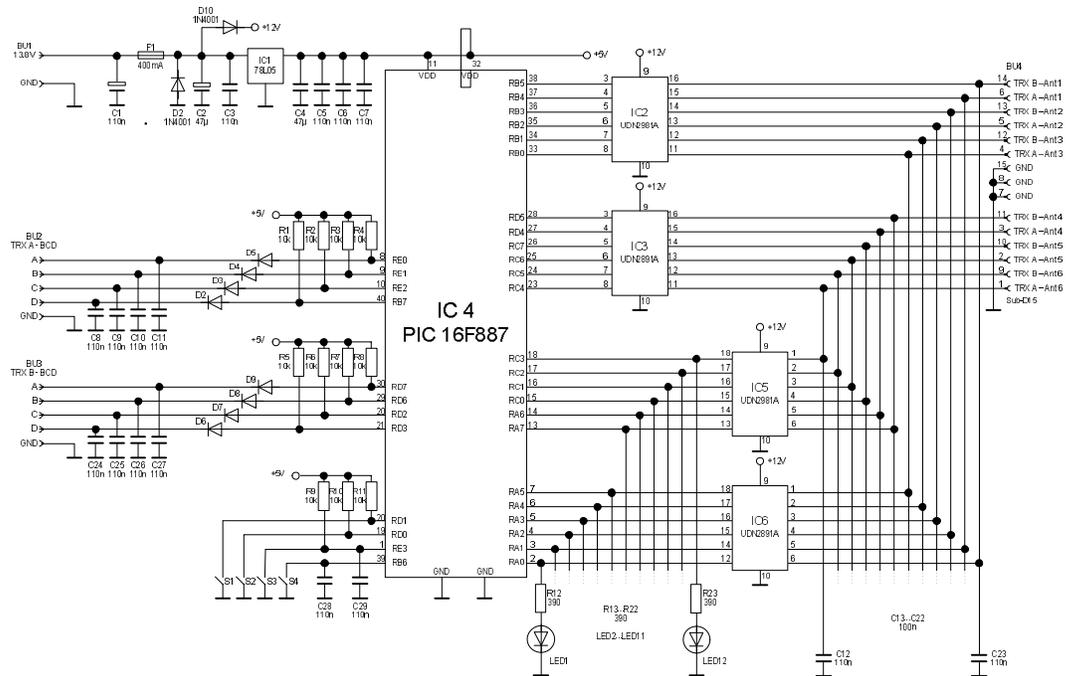
Picture 6: automatic controller for 6x2 antenna switch using BCD outputs of transceiver
