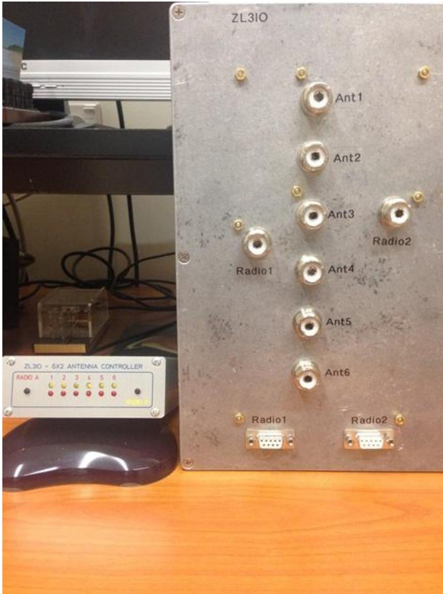
Picture 9: 6x2 antenna switch and controller
