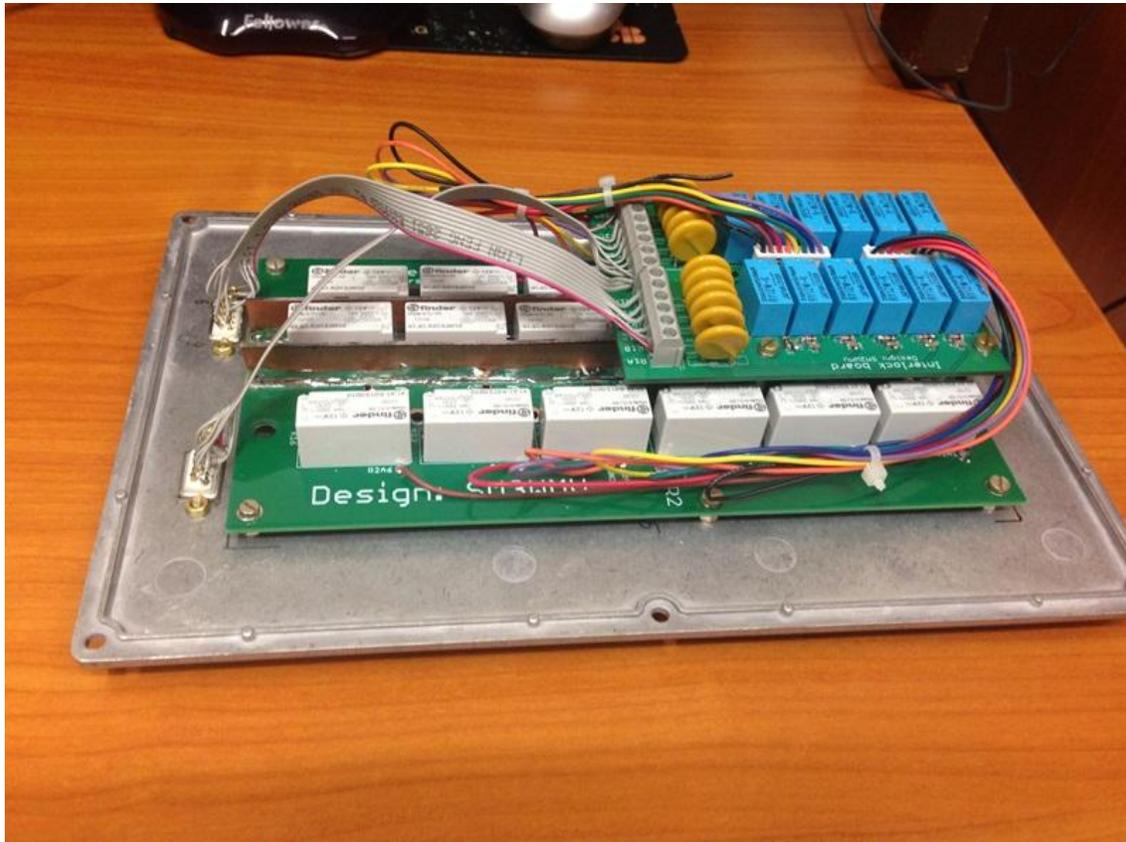
Picture 4: 6x2 antenna switch after SM2WMV, antenna relays board in the bottom and interlocking board sitting on top
