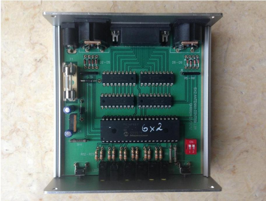
Picture 7: controller for the 6x2 antenna switch
